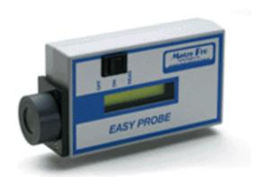
The Easy-Probe<sup>TM</sup> is a multi-lingual meter reading device that permits the reading of various electronic meters with this single device.
